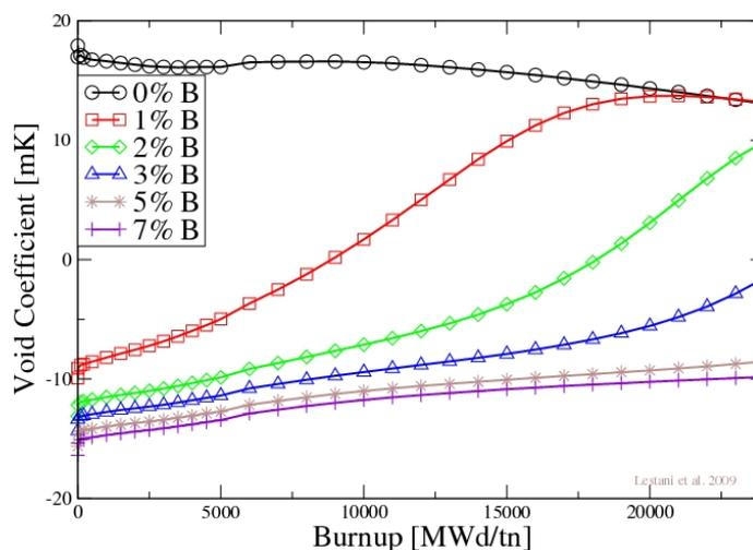
Fig. 5. Evolution of coefficient with burnup for different B contents.
