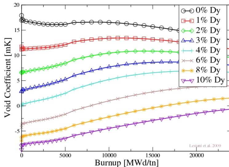
Fig. 1. Evolution of coefficient with burnup for different Dy contents
