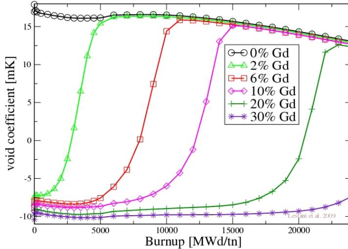
Fig. 3. Evolution of coefficient with burnup for different Gd contents.
